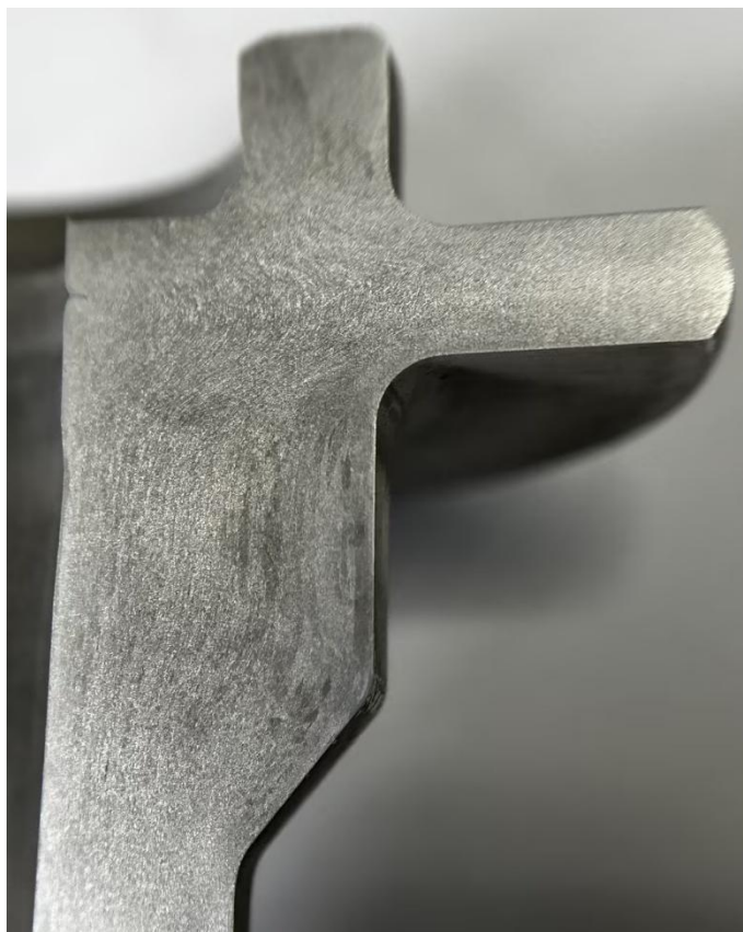
Image 3: The grain lines not broken and make the structure stronger.
